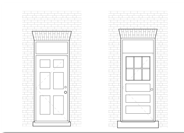
Door elevations in brick
